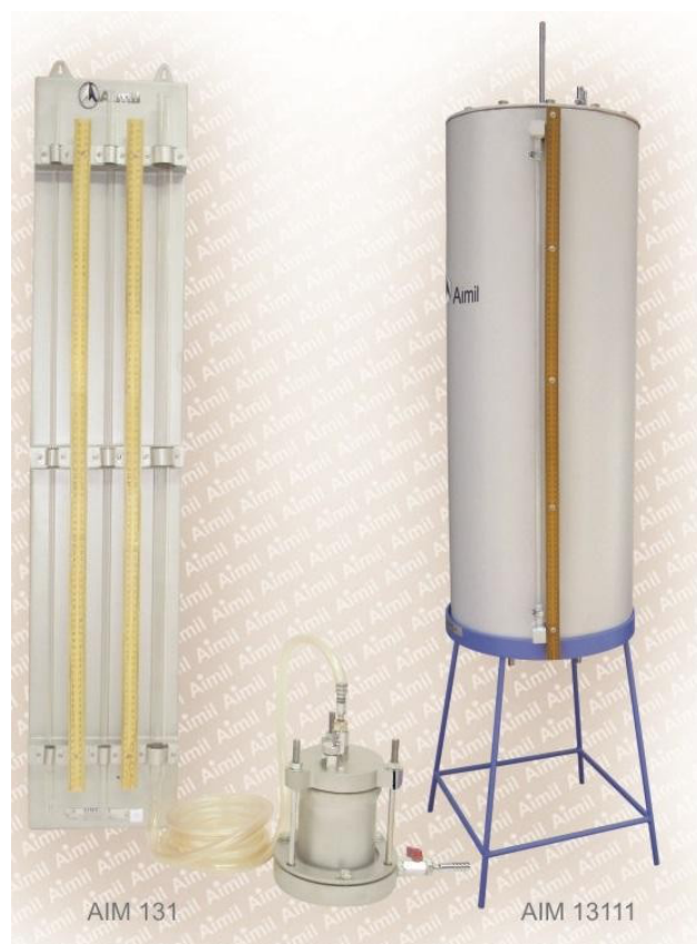
Figure 2: Laboratory Soil Permissibility Apparatus
