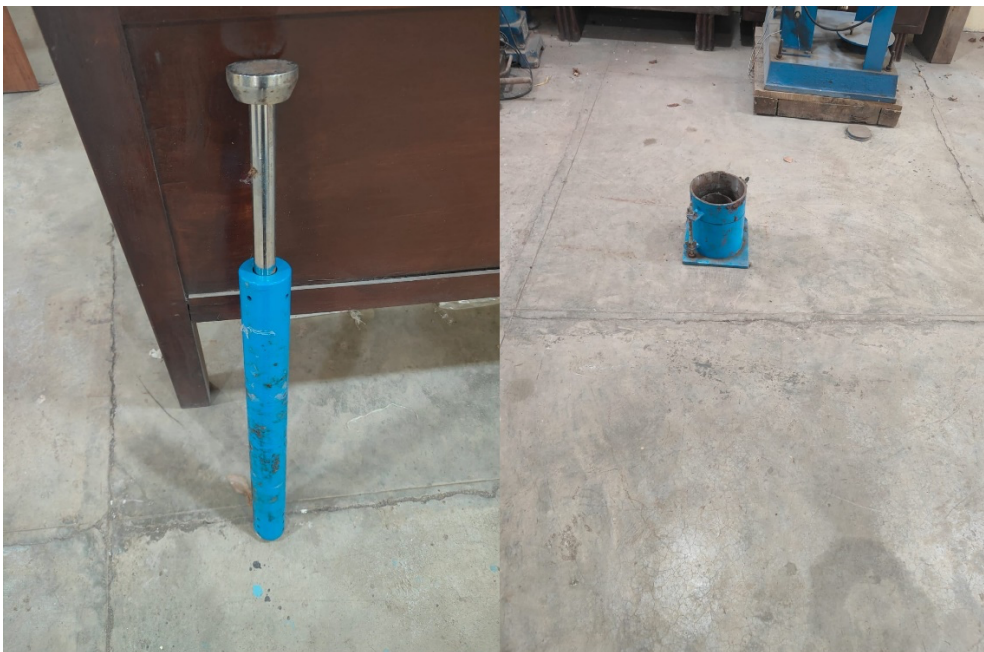
Figure 1: Soil Compaction Hammer
